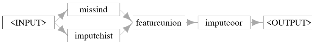
Figure 9.2: Pipeline to impute missing values of numeric features by histogram with binary indicators and missings in categoricals out-of-range with a new level.
